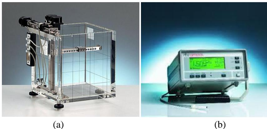
**Fig. (2): MP3 water phantom (a) and PTW-UNIIDOS electrometer (b).**
