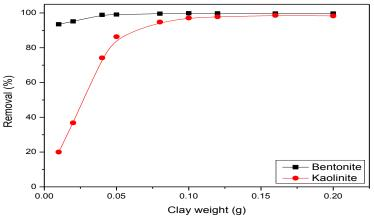
Fig. 3: Effect of adsorbent weight on the removal efficiency of Eu(III) ( $C_M = 10^{-4}M$ , pH=4,  $t_{eq}$ 60 min., temperature 298±1 K).
