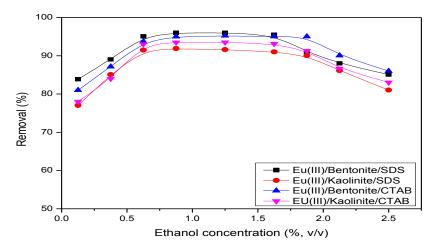
Fig. 6: Effect of ethanol concentration on the flotation efficiency of Eu(III)-loaded clays.
