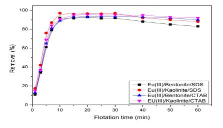
Fig. 7: Flotation of Eu(III)-loaded clays as a function in the flotation time.
