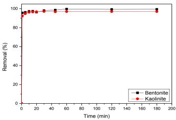
Fig. 2: Effect of contact time on adsorption of Eu(III) using bentonite and kaolinite( $C_M = 10^{-4}$  M, pH=4, clay 0.1 g, temperature 298±1 K).
