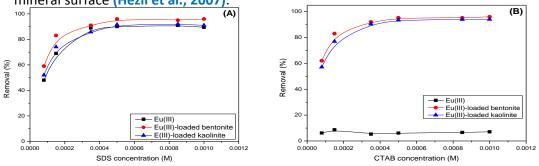
Fig. 5: Effect of collector concentration on the removal efficiency of Eu(III) by ion and sorptive flotation.
