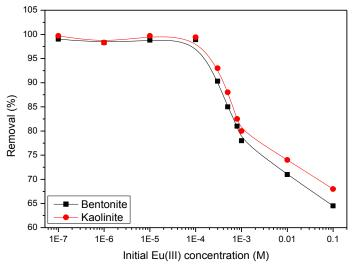
Fig. 4: Effect of initial concentration of Eu(III) on its removal percentage by the
