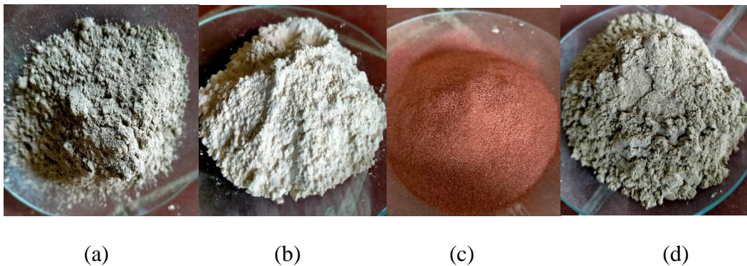
Fig.1. (a) ground granulated blast furnace slag (GGBFS), (b) metakaolin (MK), (c) ground clay brick (GCB) (d) cement kiln dust (CKD)
