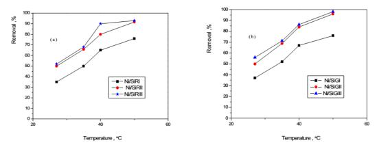
**Fig.(4)** : *Effect of temperature on the adsorption of Cr(IV) from waste water onto a) Ni/SiR and b) Ni /*SiG solids.
