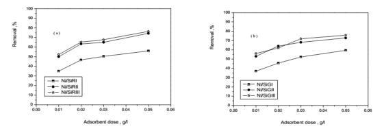
Fig.(2) : Effect of adsorbent dose on the adsorption of Cr(IV) from waste water onto a) Ni/SiR andb) Ni /SiG solids.
