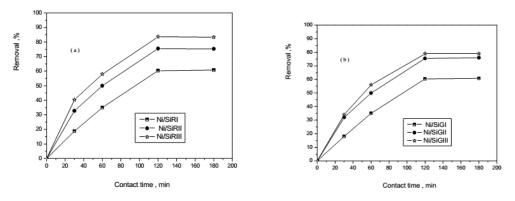
Fig.(3) : Effect of contact time on the adsorption of Cr(IV) from waste water onto a) Ni/SiR and b) Ni /SiG solids.
