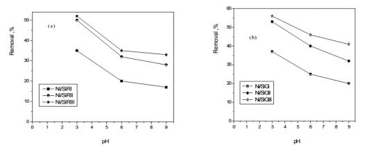
Fig.(1) : Effect of pH on the adsorption of Cr(IV) from waste water onto a)Ni/SiR andb)Ni /SiG solids.
